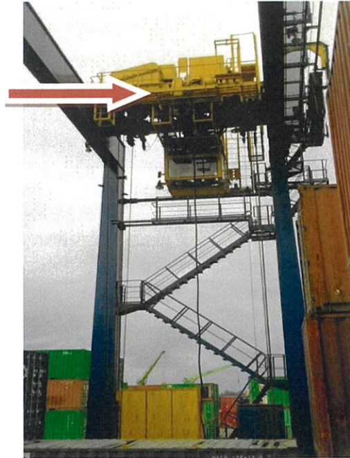
Gambar 2.6. Ruang Kontrol / Kabin Operator
