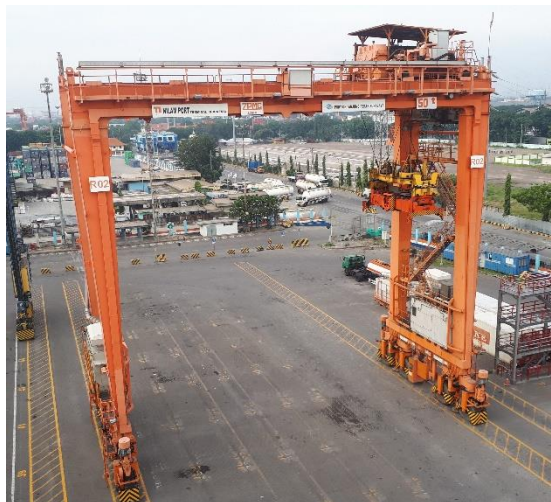
Gambar 2. 1 Unit Rubber Tyred Gantry (RTG) Sumber : PT Nilam Port Terminal Indonesia
