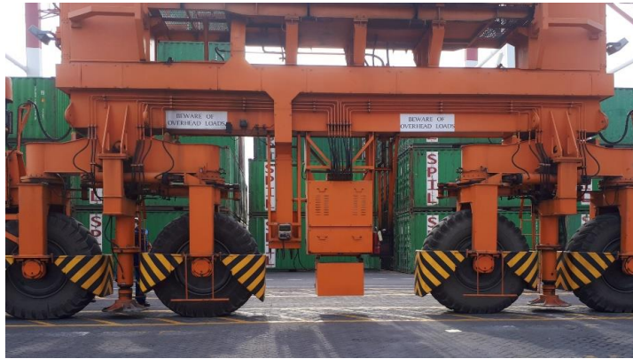
Gambar 2. 4 Bagian Bogie Area & Whell turning
