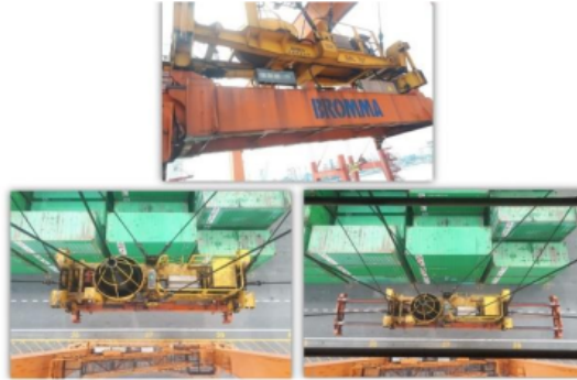
Gambar 2. 8 Bagian Spreader Telescopic Single Lift & Headblock Sumber : PT Nilam Port Terminal Indonesia
